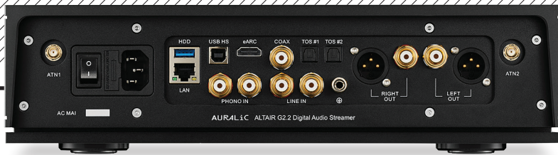
ABOVE: Wired/wireless network control/streaming supplements access to more music via internal and external (HDD) USB-A drives. A USB-B (DSD512/DXD) input is joined by 2x Toslink, coaxial and HDMI eARC alongside analogue line and phono inputs. Fixed/variable analogue output is offered on RCAs and balanced XLRs
