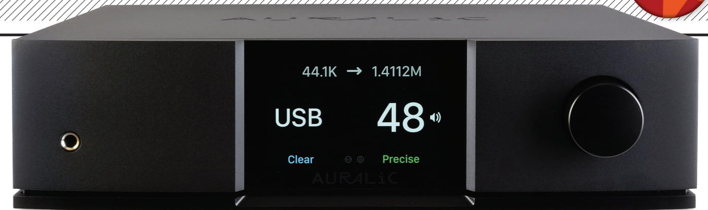
ABOVE: The 100mm TFT display allows the user to navigate the comprehensive system/setup menu and also reveals the library of albums/songs available or in play (including cover art)
